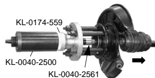
Drive-Shaft extraction with the Hydraulic Cylinder (17 t.)
