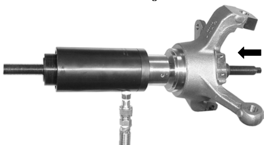
New wheel bearing insertion
