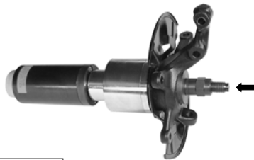
Wheel bearing extraction with KL-0040-61 A
